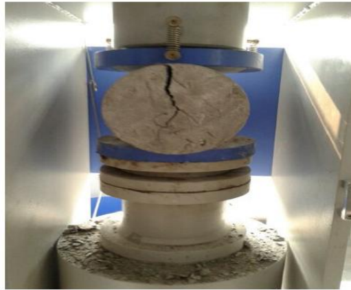
Figure 2. Split tensile strength test specimen
