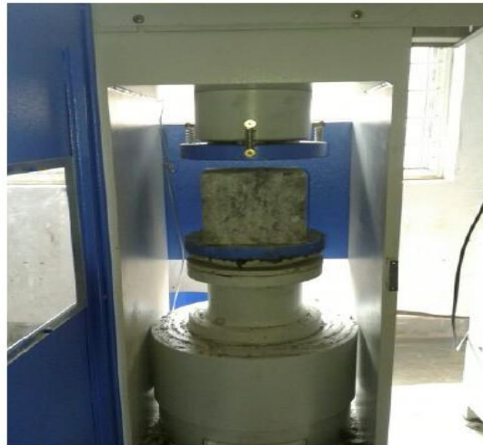
Figure1. Compressive strength test specimen
